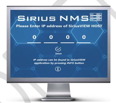
The screen above will appear whenever Sirius NMS application is executed. During run-time, if user wants to change IP address of host or wants to monitor different host, user just needs to press "ESC" button to call IP address entry window
